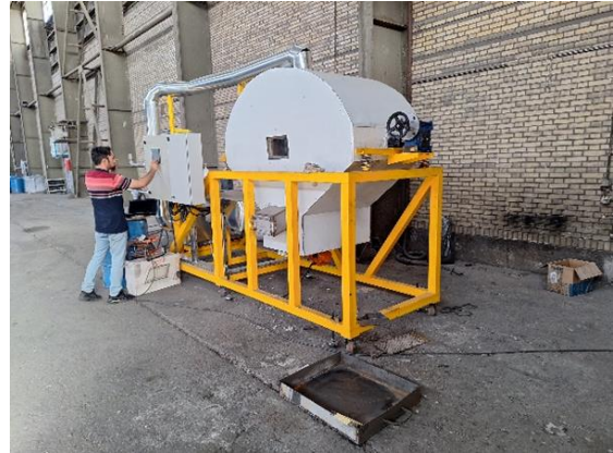
Figure 6. pilot-scale fluidized bed was constructed as part of this research.
