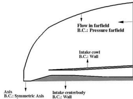
**Figure 1. The computational grid and the boundary conditions**
