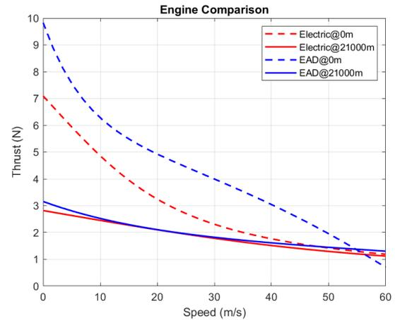
**Figure 3 – Thrust vs. Velocity for Both Propulsion Systems**
