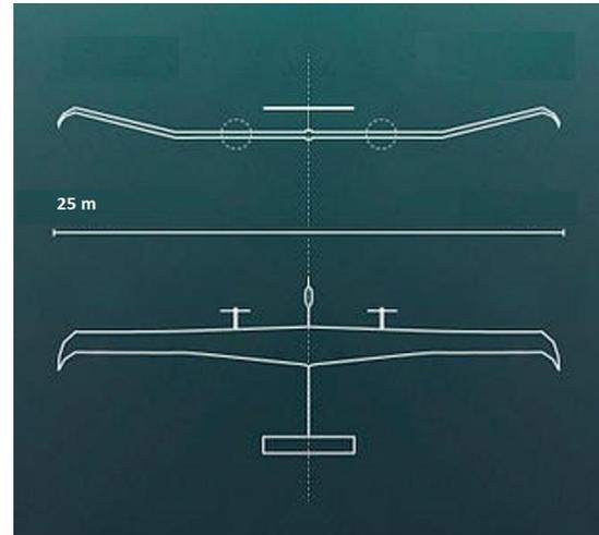
Figure 2. Schematic diagram of the Zephyr 8 unmanned aerial vehicle (UAV)
