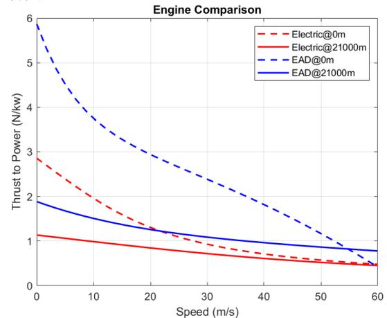
**Figure 4 – Thrust-to-Power Ratio vs. Velocity for Both Propulsion Systems**
