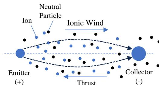
**Figure 1. Schematic illustration of ionic wind generation in an electroaerodynamic propulsion system.**
