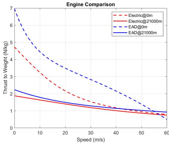
**Figure 5 – Thrust-to-Weight Ratio vs. Velocity for Both Propulsion Systems**
