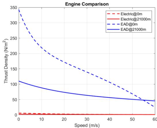
**Figure 6 – Thrust Density vs. Velocity for Both Propulsion Systems**
