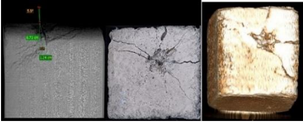
Figure 5. Sample photo after testing and scan results for a projectile with impact angle of 5 degrees and an impact velocity of 552 m/s
