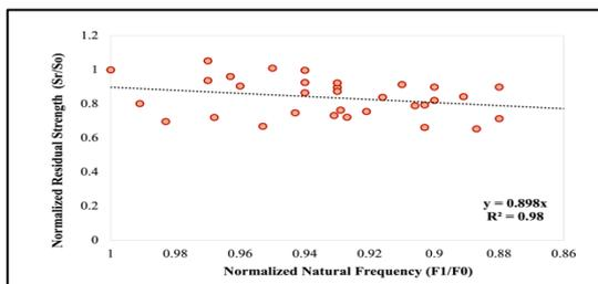
**Figure 5 - Normalized natural frequency versus normalized residual strength.**
