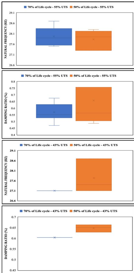
**Figure 4 – Modal analysis of samples at two fatigue stress levels for two different fatigue life.**
