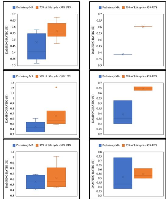
Figure 3- Damping ratio (%) variation before and after fatigue damage at two fatigue stress levels of 55 and 43%.
