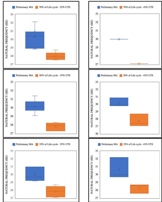
Figure 2- Natural frequency variation before and after fatigue damage at two fatigue stress levels of 55 and 43%.
