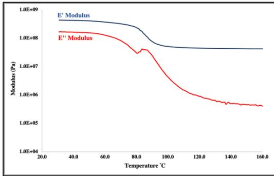
Figure 1 - Dynamic mechanical thermal analysis of GFRP including the storage and loss modulus.
