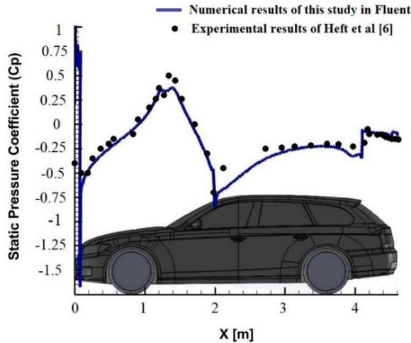
**Figure 1.** The distribution diagram of the static pressure coefficient above the standard body and comparison with the experimental results of the wind tunnel of the Technical University of Munich [6] at the Reynolds number of  $4.87 \times 10^6$
