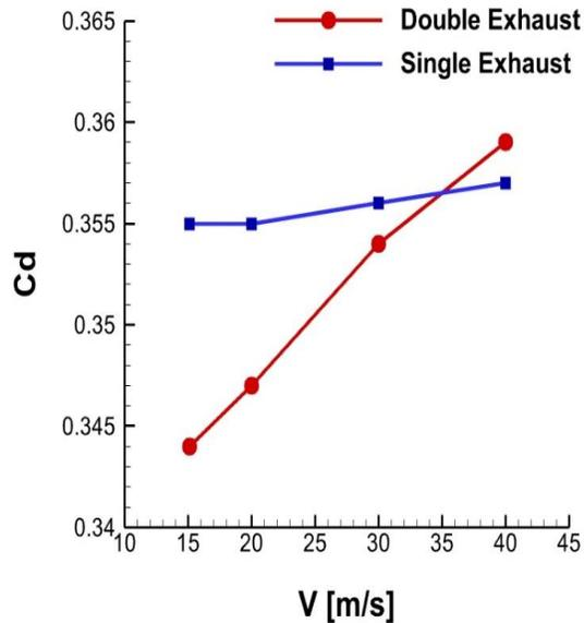
Figure 2. The comparative graph of the total drag coefficient difference for the car with dual and single exhaust systems
