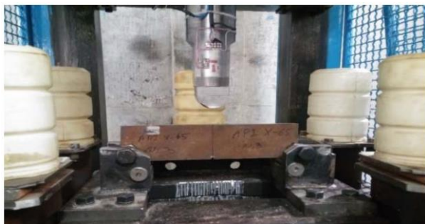
Figure 1. The Laboratory specimen in the DWTT.
