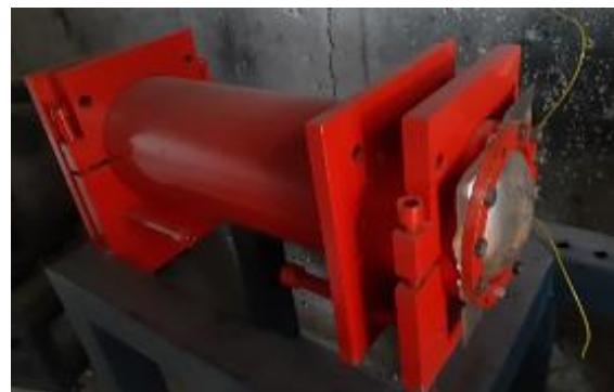
Figure 5- Sheet test with a core combination of resin and mineral pumice
