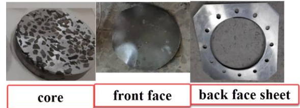
Figure 7- The result of an experiment with a core made of aluminum and pumice
