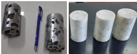
Figure 2. Foam and aluminum samples of pressure test
