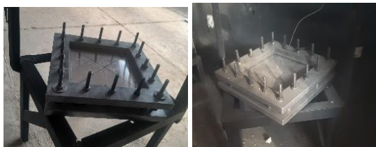
Figure 13- Sample with aluminum face sheet before and after the test
