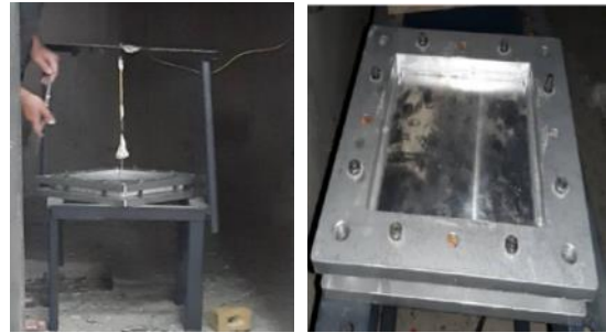
Figure 3- Free explosion test on sandwich panel
