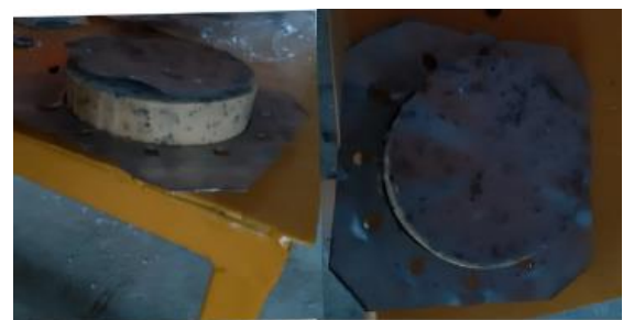
Figure 6- Sample with foam core after testing
