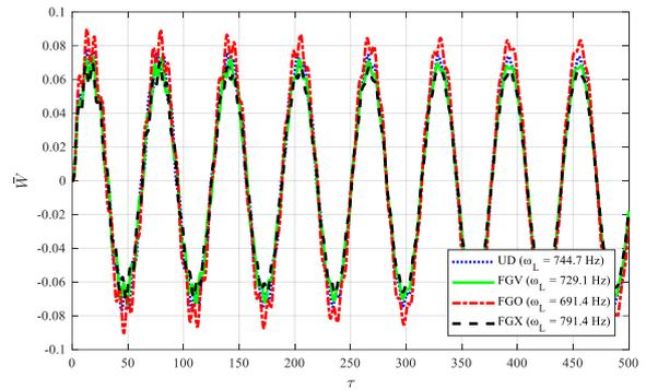
Figure 5. Distribution pattern of CNTs on nonlinear dynamic response of conical shell reinforced with CNTs
