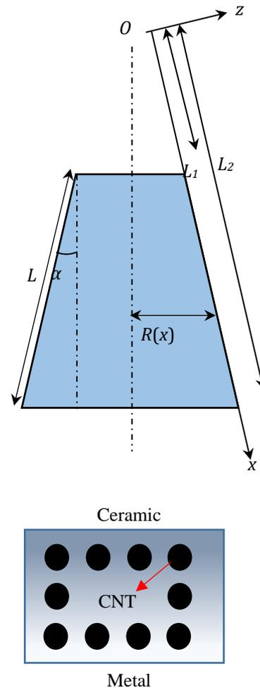
**Figure 1. Schematic of truncated conical shell reinforced with CNTs with ceramic and metal matrix**
