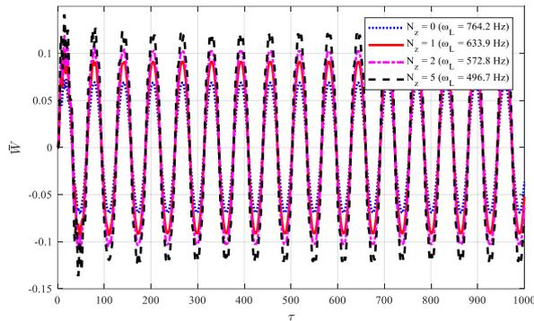
Figure 3. Effect of power index on nonlinear dynamic response of conical shell reinforced with CNTs
