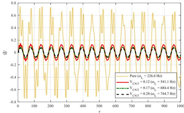
Figure 4. Effect of volume fraction of CNTs on nonlinear dynamic response of conical shell reinforced with CNTs
