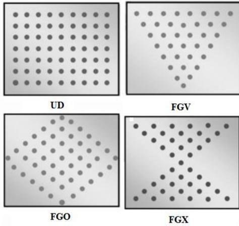
Figure 2. Types of distribution patterns of CNTs
