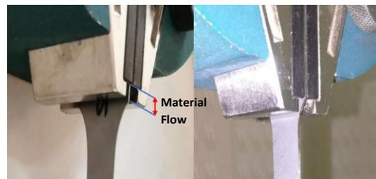
Figure 5. Flowing of material from the jaw during the test
