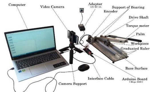
Figure 2. The experimental setup used to measure the jamming-in travel
