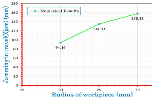
Figure 3. Numerical results of jamming-in travel of workpieces with different diameters
