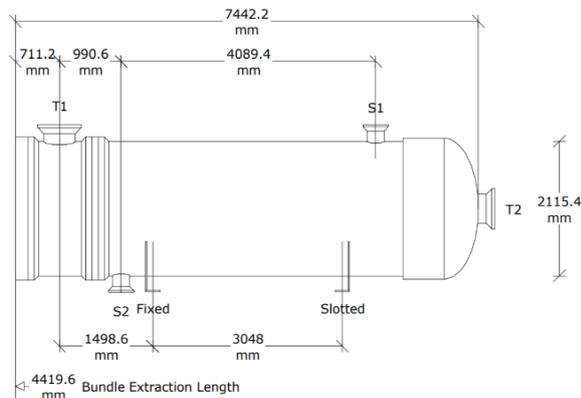
Figure 1. The heat exchanger used in the present work [12, 13]
