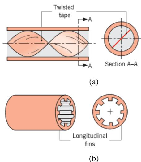
Figure 2. Geometry of turbulators used in the present work (a) twisted tape and (b) microfin [14]
