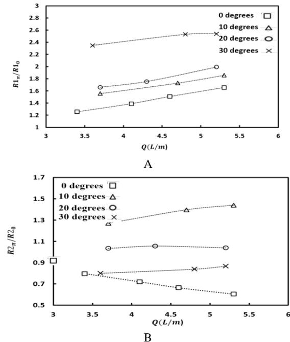
Figure 3. (A) Variations of the  $R_{1\pi}/R_{1_0}$  to flow rate for different nozzle angles 2, (B). Variations of  $R_{2\pi}/R_{2_0}$  to flow rate for different angles of nozzle 2 ( $S/D = 20$ )
