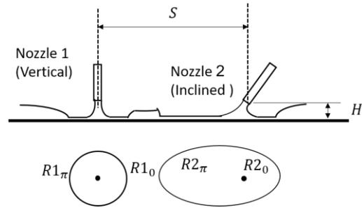
**Figure 1 - Schematic of hydraulic jumps created by two impinging inclined and vertical jets on a surface**
