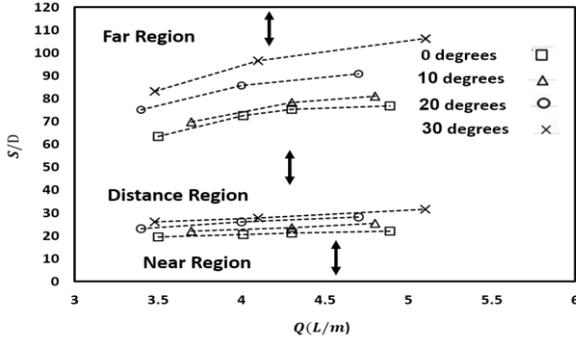
Figure 2 - Effect of the inclination angle of a nozzle on the boundary of the regions formed by the jumps of two fluid jets
