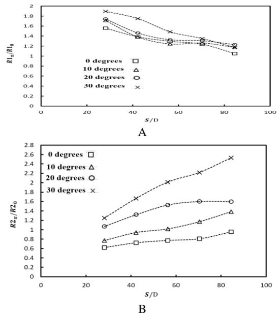
Figure 4. (A) Variations of  $R_{1\pi}/R_{1_0}$  to  $S/D$  for different angles of nozzle number 2, (B). Variations of  $R_{2\pi}/R_{2_0}$  to  $S/D$  for different angles of nozzle number 2 ( $Q = 4.4$  Lpm)
