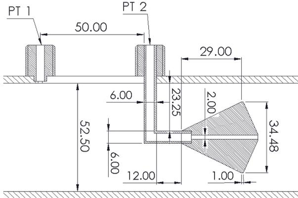
**Figure 1. Geometry of continuous nose V-Cone flowmeter (all dimensions are in mm)**
