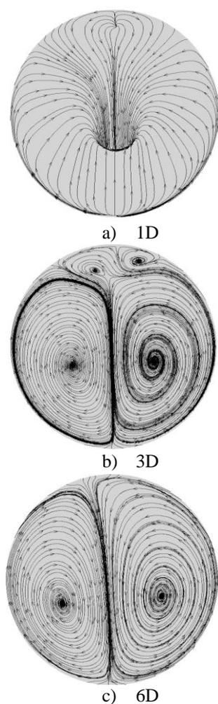
**Figure 2.** Flow streamlines in the  $y$ - $z$  plane and for  $Re=9.2 \times 10^4$
