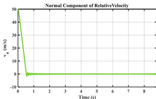
Figure 7. The relative speed of the missile and the target - SMC-NN controller
