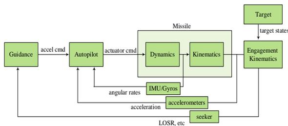
Figure 1. Block diagram of three-loop autopilot
