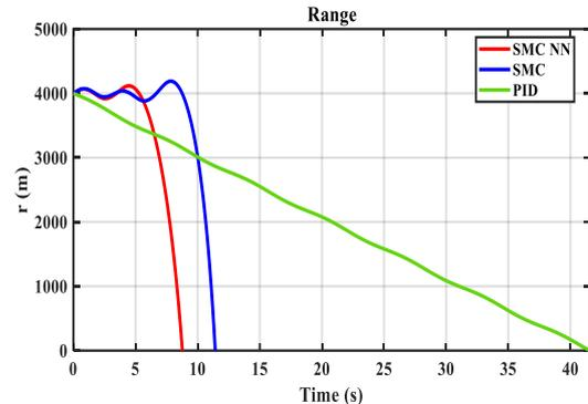
Figure 8. The relative distance between the missile and the target
