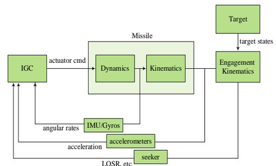
Figure 2. Block diagram of Integrated Guidance and Control (IGC)
