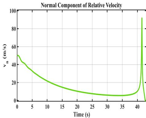
Figure 5. The relative speed of the missile and the target - PID controller
