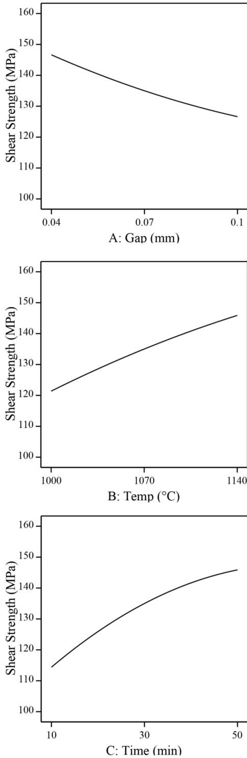
**Figure 2. Effect of joint seam, temperature and time on shear strength of joints**
