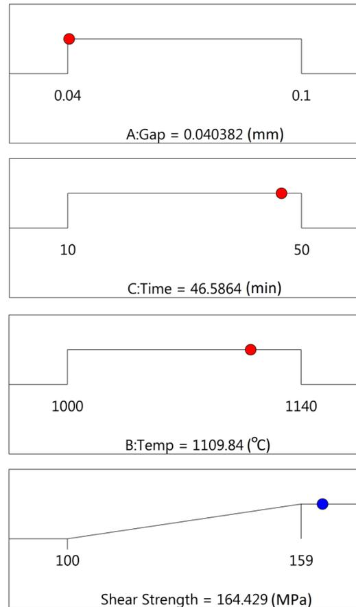
**Figure 3. The optimization results using the response surface methodology**
