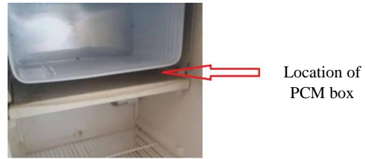
(b) Figure 1. (a) Ordinary refrigerator-freezer (b) Placement of PCM slab
