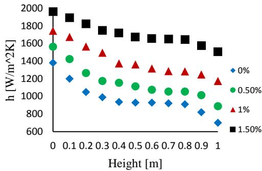
Figure 3. Heat transfer coefficient for various concentrations at a Reynolds number of 4200
