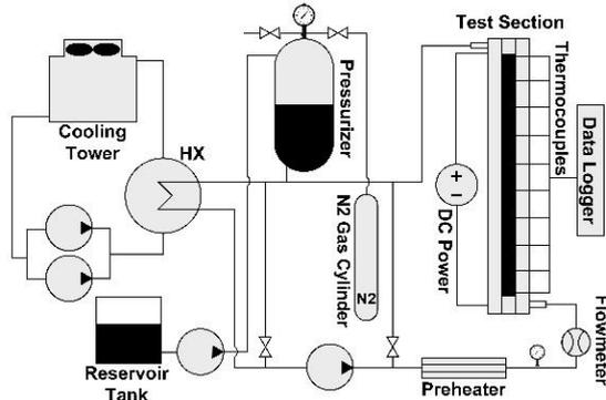
Figure 1. Schematic picture of the test loop
