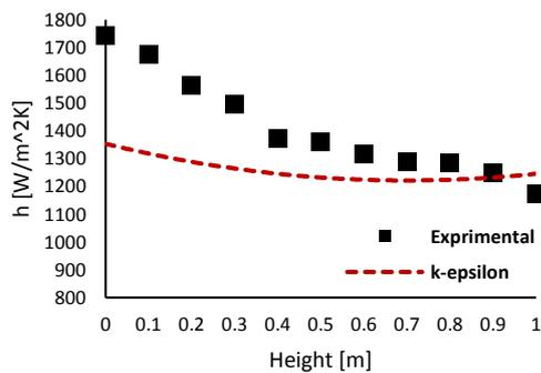
Figure 4. Heat transfer coefficient of nanofluid 1% at a Reynolds number of 4200
