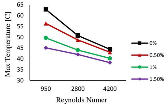
Figure 2. The maximum temperature of the rod at various Reynolds numbers and concentrations
