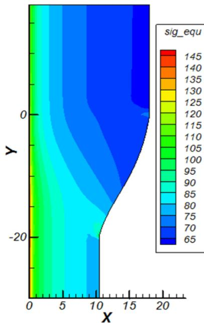
Figure 2 - Distribution of Von Mises Stress in MPa during Material Extrusion in the Optimal Die Shape
