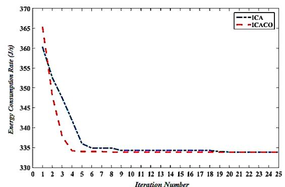
**Figure 1 - Convergence Plot for Optimal Die Shape using Hybrid Imperialist Competitive Algorithm-Ant Colony Optimization (ICA-ACO) and Imperialist Competitive Algorithm (ICA) Methods**
