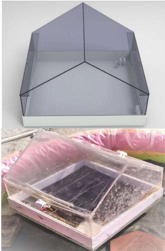
Figure 1. A view of the floating solar still
