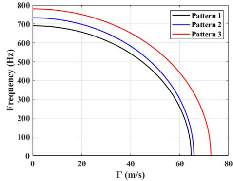
**Figure 3.** The effects of various porosity distribution patterns on the nonlinear frequency in terms of fluid velocity
