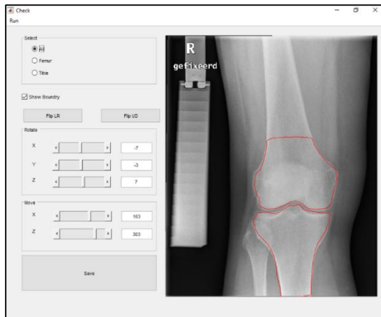
Figure 1: Displaying the boundaries of the STL files for the bones within the generated GUI environment.
