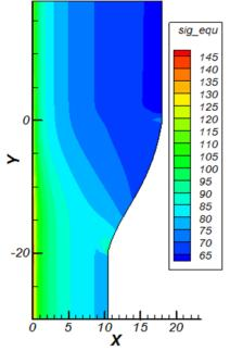
Figure 2 - Distribution of Von Mises Stress in MPa during Material Extrusion in the Optimal Die Shape
