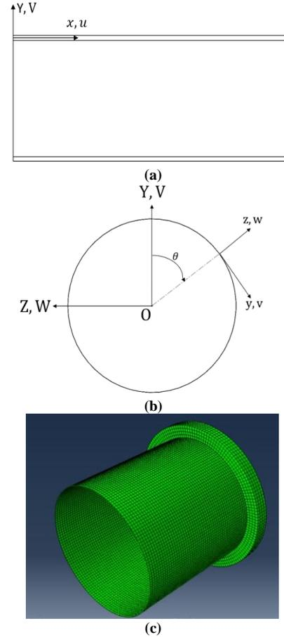
**Figure 1. The schematic of the cylindrical shell with the adopted coordinate systems (a) Side view (b) Front view (c) 3D view**
