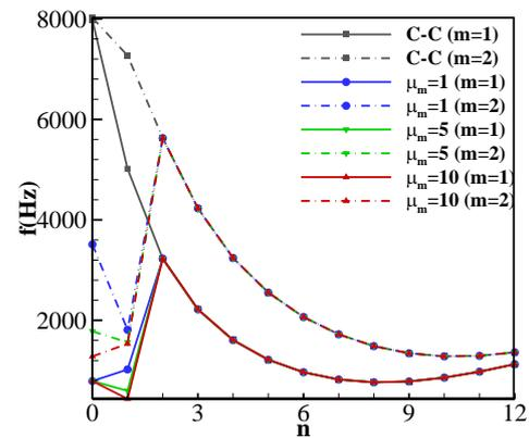
**Figure 3. Variation of the first two frequencies with  $n$  obtained for three different disk masses**
