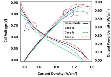
Figure 3. Polarization curves of different models
