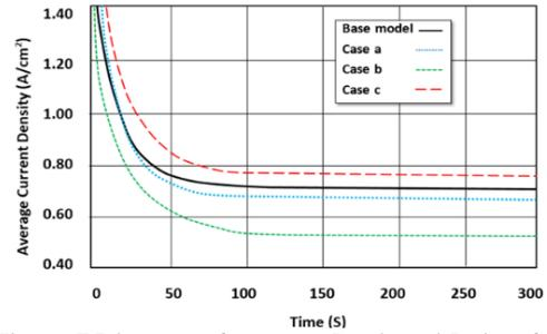
Figure 7. Diagram of current density with time for different models
